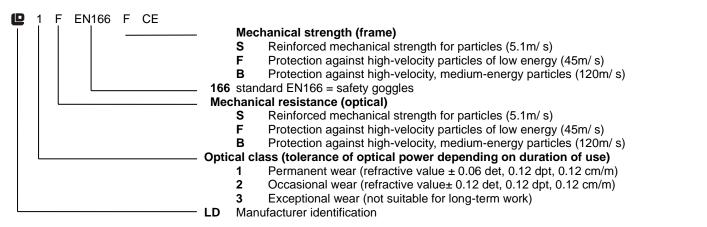
If the symbols S, F and B are not common to the eyepiece and frame, then the lowest level should be assigned to the full eye protector. The letter T immediately after the impact symbol authorises use for particles launched at high speed at extreme temperatures. If the letter T is not present, the protector should be used at room temperature.
