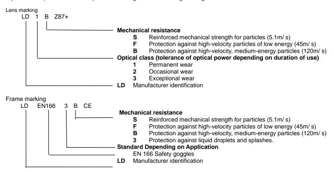
If the symbols S, F and B are not common to the eyepiece and frame, then the lowest level should be assigned to the full eye protector. The letter T immediately after the impact symbol authorises use for particles launched at high speed at extreme temperatures. If the letter T is not present, the protector should be used at room temperature.
