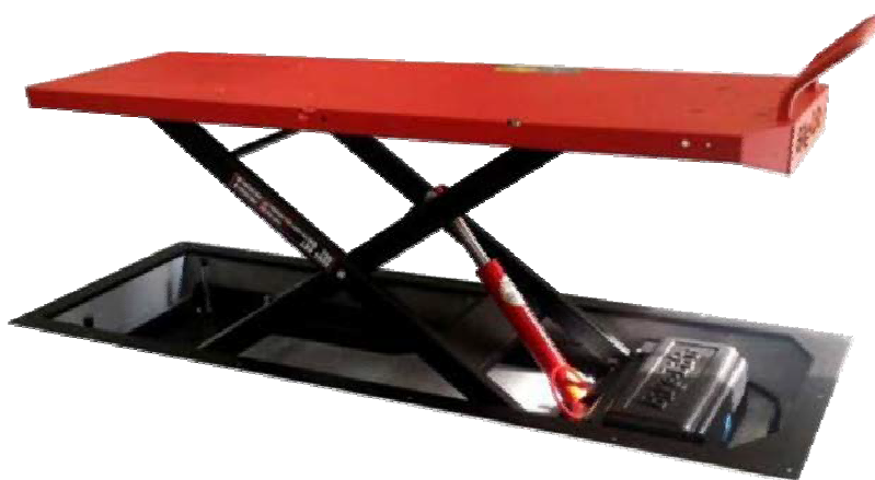
Figure 4 - Example of a built-in lifting platform
