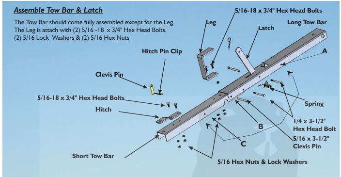
To fold Tow Bar up, into the push location: First pull the Hitch Pin Clip from the 5/16 X 3-1/2" Clevis Pin, pull out the Pin From hole (B) and fold the Short Tow Bar under the Long Tow Bar. Line up hole (C) with hole (A), push Pin through (A) &(C) and replace the Hitch Pin Clip.
