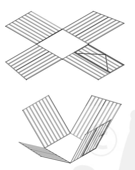
**Step 2.** Raise the panels in sequence as shown. The side panels will rest in the cut-out section of the front and rear U channels. Working from outside the shed, fasten the screws through the corner rib overlap.
