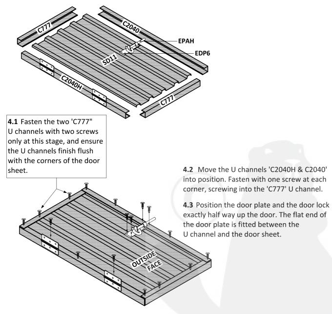
**4.4** Check that all the U channels are located correctly, and are parallel with each other, then continue to fasten all the components together as shown above.
