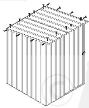
**Step 5.** Secure the shed to the concrete in accordance with the recommendations on page 7. If the site or concrete slab is not quite level, as often happens, the door may not align with the jambs properly. This may be adjusted by levering under the wall and packing beneath it, either directly below the bolt or below the hinges. A trial will soon show which is required. This adjustment should be made before anchoring the shed.
