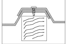
Hold a small block of timber under the bottom sheet to support the drilling pressure, allowing the screw to quickly drill and fasten the second sheet.
