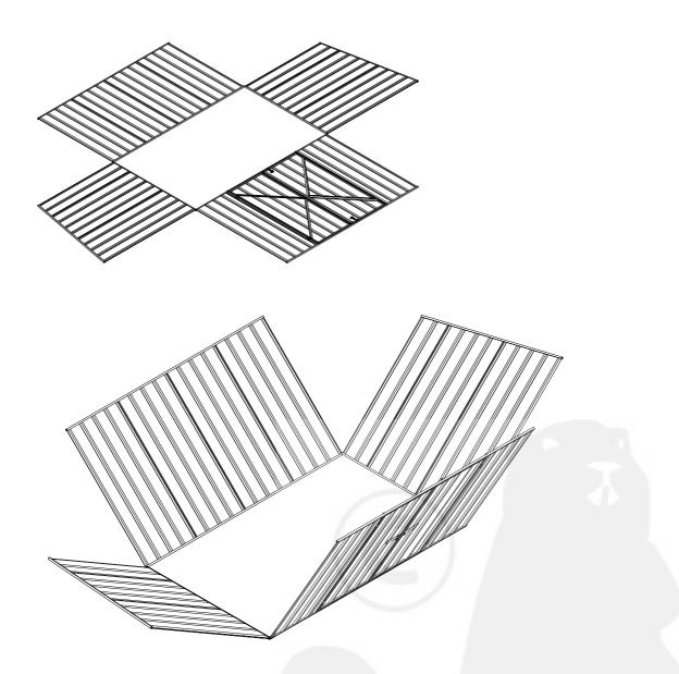
**Step 2.** Raise the panels in sequence as shown. The side panels will rest in the cut-out section of the front and rear U channels. Working from outside the shed, fasten the screws through the corner rib overlap.
