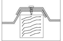
Hold a small block of timber under the bottom sheet to support the drilling pressure, allowing the screw to quickly drill and fasten the second sheet.
