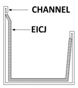
The channel joiners 'EICJ" supplied fit neatly inside the channels to be joined together, without the need for screws. Ensure that half of the 220mm long channel joiner is allocated to each channel when they are butted together. Handle these joined channels carefully until they attain full strength after being fastened to the roof and wall sheets as noted on following pages.
