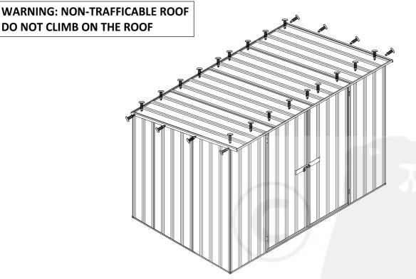
**Step 5.** Secure the shed to the concrete in accordance with the recommendations on page 7. If the site or concrete slab is not quite level, as often happens, the door may not align with the jambs properly. This may be adjusted by levering under the wall and packing beneath it, either directly below the bolt or below the hinges. A trial will soon show which is required. This adjustment should be made before anchoring the shed.
