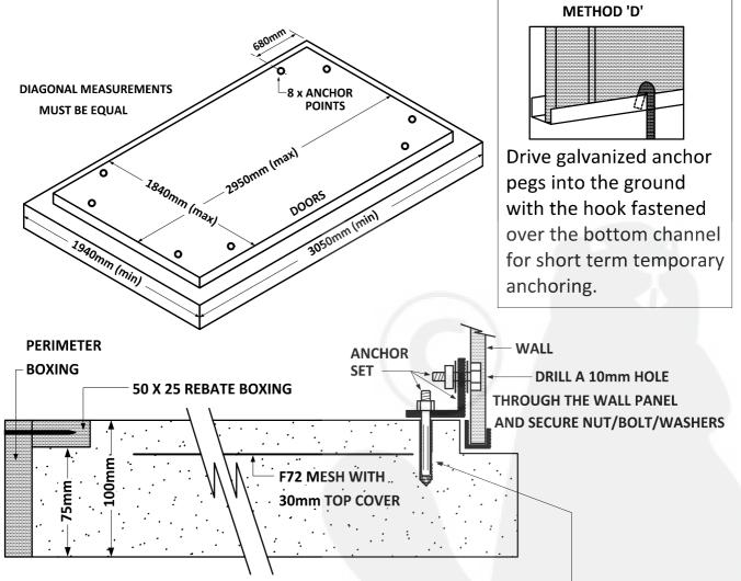
Using a 10mm diameter masonry drill, position the bracket and drill a 60mm deep anchor hole in the concrete. Insert the masonry anchor through the bracket into the anchor hole until the anchor nut is firmly seated against the bracket. Tighten the anchor nut with a spanner to attain maximum strength.
