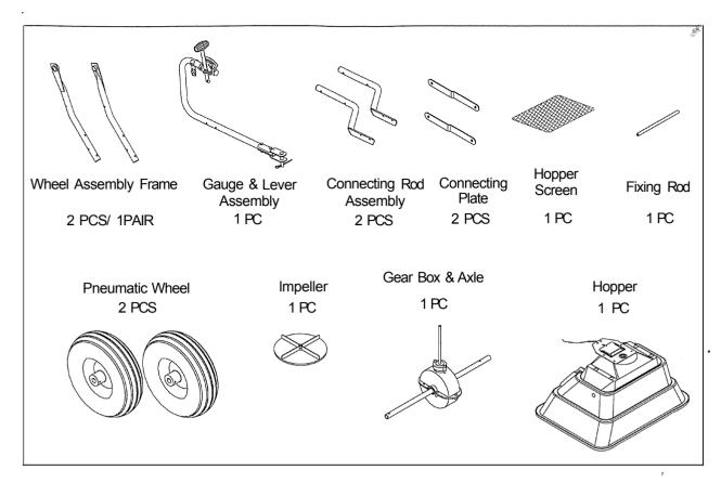
STEP1 : Install Impeller onto the Gear Box & Axle Assembly. Insert Round Head Bolt M4x20 through impeller then through Gear Box Axle.
