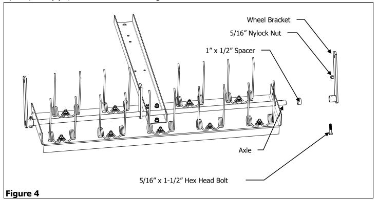
5. Place a 1/2" Flat Washer onto a 1/2" x 3" Hex Head Bolt, followed by a Wheel and then another 1/2" Flat Washer and secure with a 1/2" Jam Nut (Do not over tighten or the Wheel will not turn). Insert this assembly into the hole in the Wheel Bracket, then secure with a 1/2" Nylock Nut. Repeat
