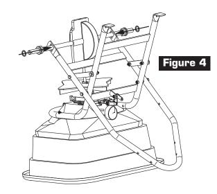
4. Install both Axle Bearings into the square holes as shown in Figure 4. Install one Washer onto each side of Axle.
