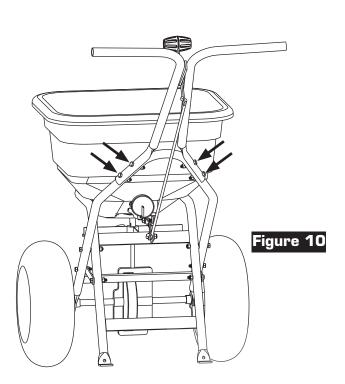
Attach Handle Assembly to Frame using (4) 1/4 x 1-3/4" Bolts and 1/4" Nylon Locknuts as shown in Figure 10.
