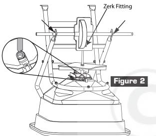
Insert Axle Assembly into the square holes on the Axle Support as shown in Figure 2.
