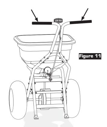
11. Install Handle Grips on Handles of Spreader as shown in Figure 11.
