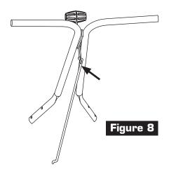
8. Install Linkage to Lever as shown in Figure 8.
