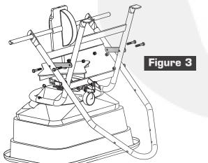
Align the Cross Braces to the Hopper and Axle Supports as shown in Figure 3. Using (4) 1-1/2" Bolts and Nylon Locknuts, assemble Cross Braces. Tighten Cross Brace Bolts securely.
