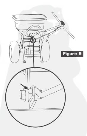
9. Turn Handle Assembly sideways and install Linkage into Rate Gate Lever as shown in Figure 9.
