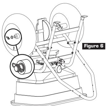
6. Install Wheel on the opposite side of the Axle (valve stem out) until it touches Axle Bearing and Washer.
