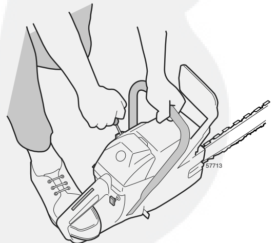
Figure 4.13 Testing the Starter
