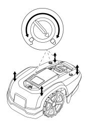
Rotate the knob to the unlock position and lift firmly at one of the corners of the body and repeat for all four corners, until the body pops loose from the chassis.
