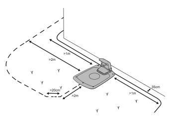
Run the guide wire to the loop on the boundary wire where the guide wire is to be connected.
