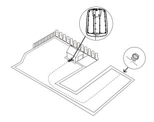
The mower uses the optional guide wire to find its way back to the charging station, but also find hard-to reach areas of the operating area. For example, the guide wire is laid between the charging station and a remote part of the working area or through a narrow passage.
