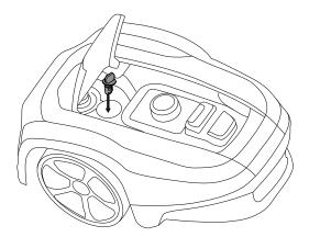
Insert the safety key into the mower and turn to the ON" (  $\mbox{\sc I}$  ) position.
