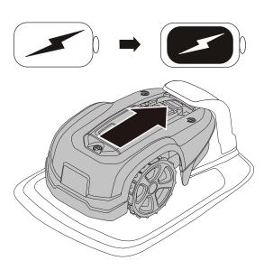
Place the mower into the charging station while the boundary and guide wires are being laid.
