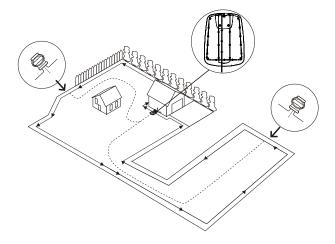
Insert both ends of the boundary wire as well as the end of the guide wire into the splice and guide wire connector. Check that the wires are fully inserted into the splice and guide wire connector so that the ends are visible through the splice and guide wire connector.
