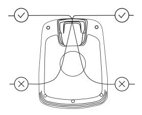
The entire charging station must be inside the operating area as shown in the figure.
