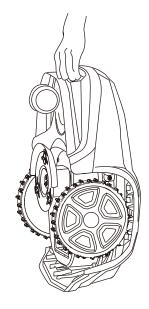
Press the STOP button and remove the safety key before lifting.
