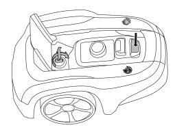
Press the **STOP** button on the mower and remove the safety key.
