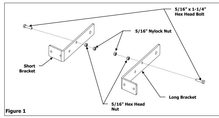
1. Insert a 5/16" x 1-1/4" Hex Head Bolt into the top center hole of both the Short and Long Brack-
