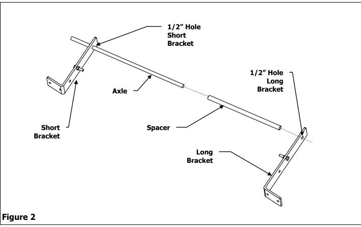
the Axle into the 1/2" hole of the Long Bracket. Centering the Brackets and Spacer on the Axle. See Figure 2.
