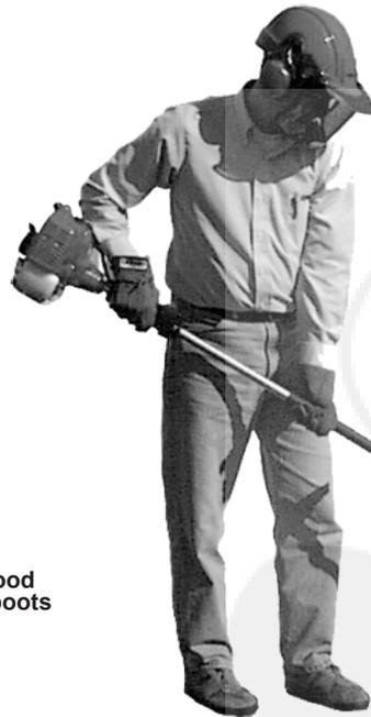
Keep bystanders at least 15 meters away from the operating trimmer to reduce the risk of being struck by falling objects or thrown debris.
