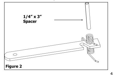
3. Slide the Latch, Spring and Spacer through the Tow Bar. This will cause the Spring to open. See Figure 3.
