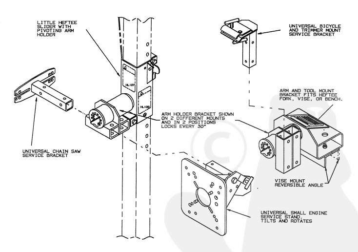
EACH SERVICE BRACKET MOUNTS ONTO THE ROTATING ARM HOLDER. THE ARM HOLDER MOUNTS ONTO EITHER THE 'LITL' HEFTEE OR THE FORK - VISE - BENCH MOUNTING BRACKET
