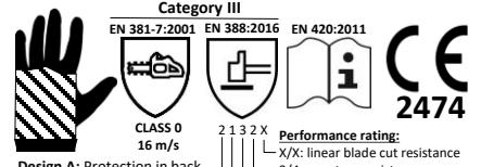
Design A: Protection in back of left glove only. No protection in fingers or thumb.
