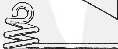
No. 2 F-436 Torsion Spring Agitator
