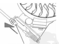
Brake lever cable adjustment
