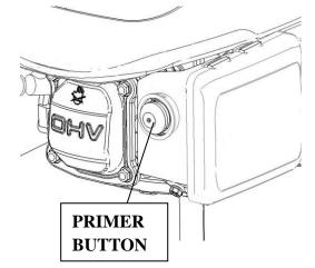
We also should put more fuel to mix air for easy start. When you push the primer button, it will pump the fuel direct from carburetor to burning house.
