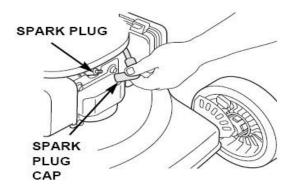
• Remove the spark plug with a spark plug wrench.
