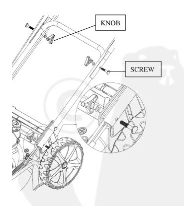
If you want to adjust height of the handle bar, you can choose" L" or "H" two holes in left-right Bracket to fix the handle bar with screws and knobs.
