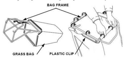
• Lift the rear discharge guard, remove the mulching plug, and install the grass bag.
