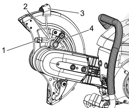
1. Raccord de tuyau 2. Tuyau
