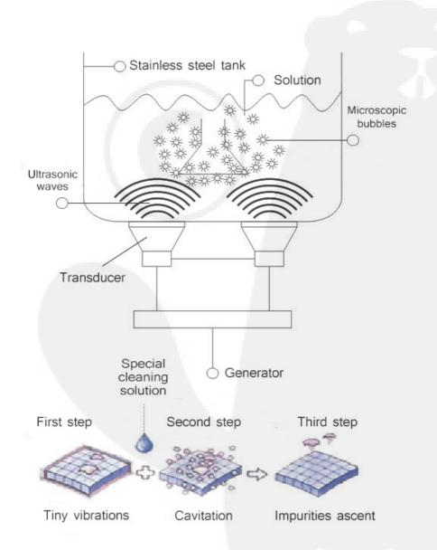
Thanks to ultrasound cleaning, we can have highest results than a basic manual cleaning. Coming from an industrial process to clean mechanical products before painting or treatment, ultrasounds cleaning is now available for many professional workshop, thanks to 2, 6 and 20 liters compact models.
