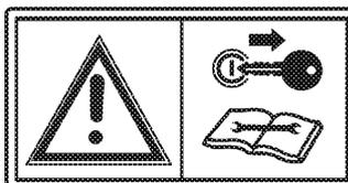
Pull the ignition plug out before maintenance and repair work.
